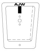
20 ga. deep drawn stainless steel cup, able to accommodate locks. 14 ga. stainless steel lifting trigger. Padlock eye to accommodate 5/16" diameter padlock shackle. Three point latch mechanism, engaging the frame at (3) points on doors greater than 42" in height; (2) engaging points on all other doors.
