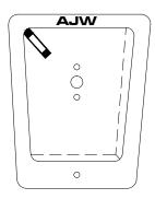
20 ga. deep drawn stainless steel cup, able to accommodate locks. 11 ga. steel hook with padlock hasp welded to door frame. Padlock hasp protrudes through stainless steel cup.
