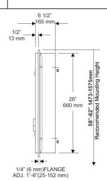
**Door**: Fabricated of type 304 #18 ga stainless steel with #4 satin finish. Door has 1/2" returns for rigidity.
