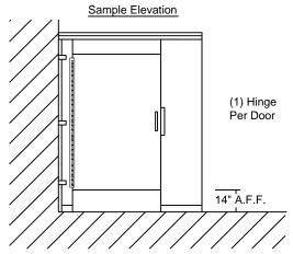
Note: Zero Degree & 20 Degree hinges are two separate items. They are not field adjustable.
