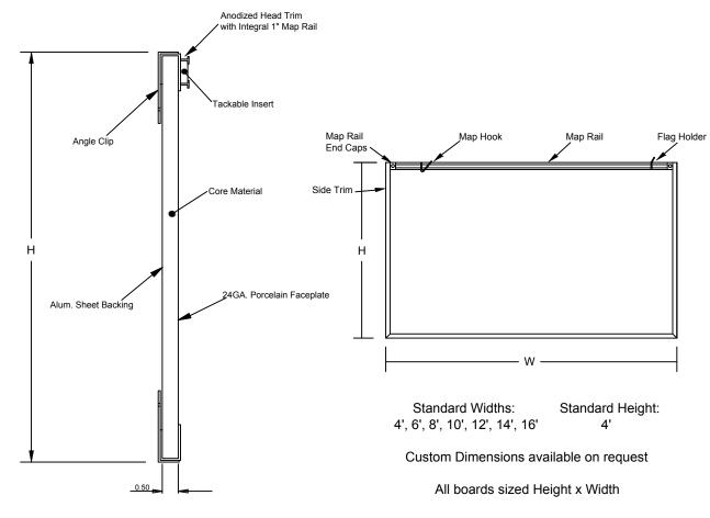
Drawing is for assembly description only. Components are not to scale for clarity purposes.
