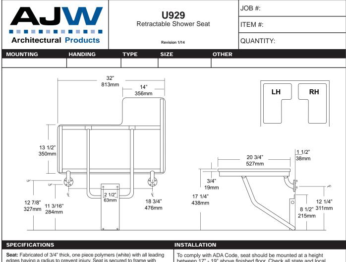
edges having a radius to prevent injury. Seat is secured to frame with carriage bolts and acorn nuts. Seat is reversible and handing is not required
