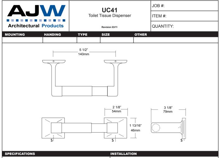
**UC Accessories:** All accessories are fabricated of high polished chrome plating over virgin zinc die cast. All UC items comply with standard federal specifications.
