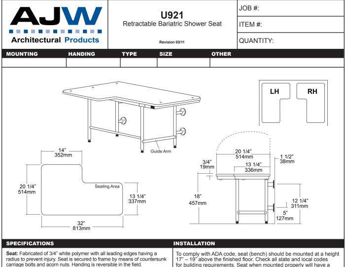
**Tubing:** Fabricated of #18 gauge stainless steel with a #4 satin finish. **Main Frame:** Fabricated of #18 gauge stainless steel, with satin finish, 1
