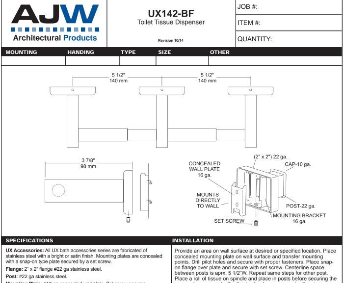
Mounting Plate: #16 ga concealed wall plate. Set screw secures mounting plate and flange.
