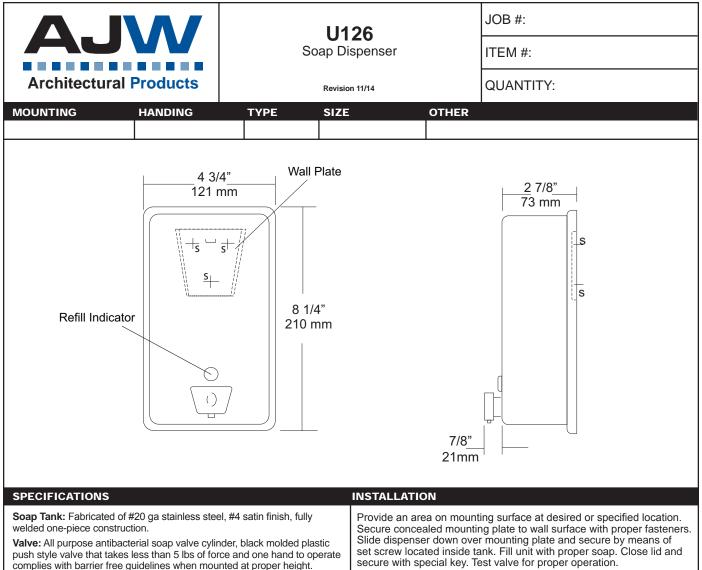
Viewer: Clear plastic window allows a constant fluid level check.
