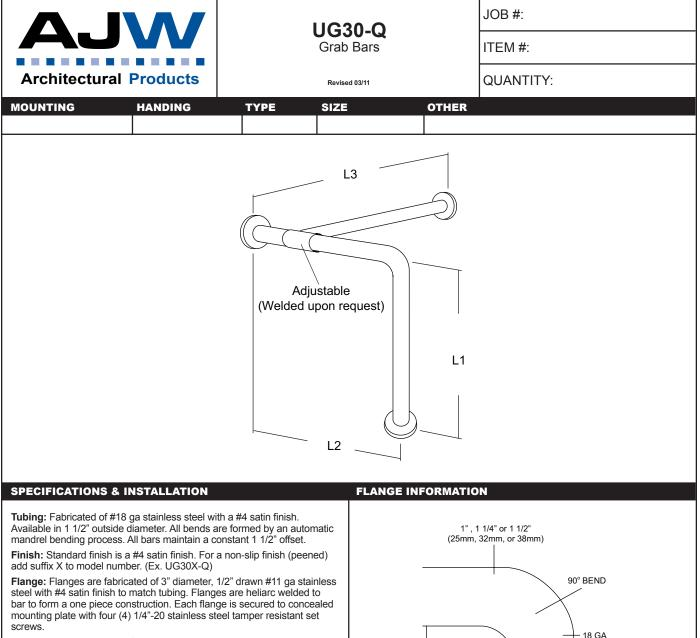
**Strength:** Bars with a 1 1/2" offset clearance will support loads in excess of 900lbs when properly installed. Bars with greater offsets will support loads up to 250lbs when properly installed.
