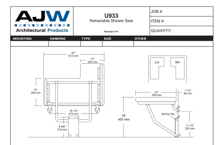
**Seat:** Fabricated of 2 1/2" thick, water-resistant reinforced vinyl fabric cushion (white) seamless design with all leading edges having a radius. Seat is secured to a 1/2" thick marine plywood.
