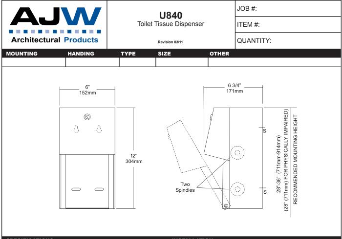
**Body:** Fabricated of #22 ga stainless steel with #4 satin finish. Concealed inner dispensing mechanism is #18 ga stainless steel.
