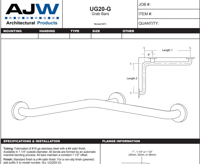
**Flange:** Flanges are fabricated of 3" diameter, 1/2" drawn #11 ga stainless steel with #4 satin finish to match tubing. Flanges are heliarc welded to bar to form a one piece construction. Each flange is secured to concealed mounting plate with four (4) 1/4"-20 stainless steel tamper resistant set screws.
